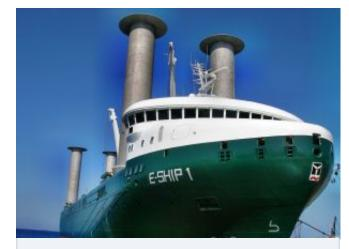
The E-Ship applies the Magnus Effect principles using the Flettner rotor, on which the Magnuss system is based; Magnuss, however, claims that its VOSS offers significant improvements
